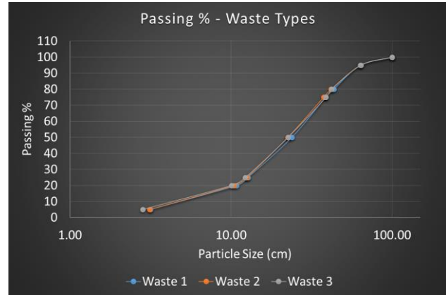
Figure 1. PSD profile for fragmentation analysis of 178 blasting events in open pit mining operations
