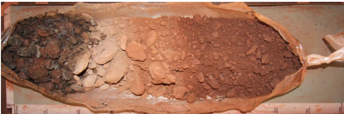
Fig. 1. Typical drill core from waste rock dump investigation
